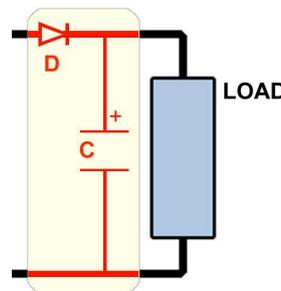
**Figure5** – Hold-up circuit on the input of each LOAD.
