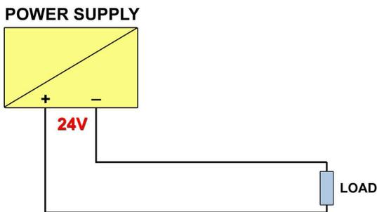
Figure1 – A power supply with a load
