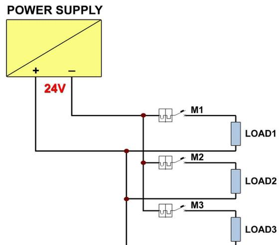
Figure3 – A power supply with more individual loads and circuit breakers for each load.
