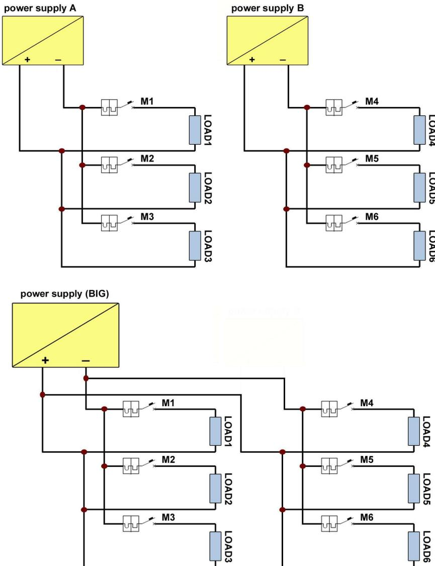
*Figure6b – Two power supplies give power to 3 LOADs each: in case of failure (short) on a LOADs, you can have only a disservice on the power of that small group*
