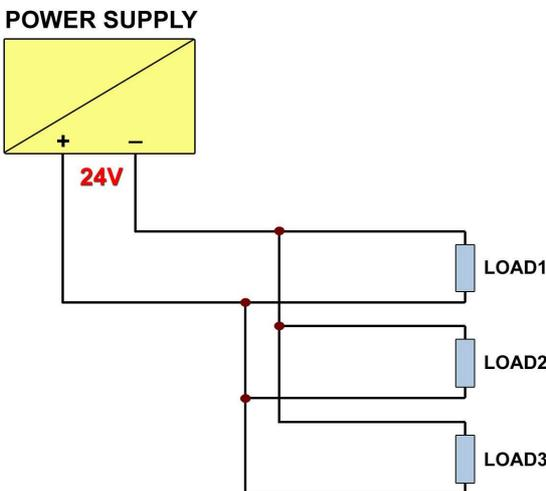
Figure2 – A power supply with more individual LOADs
