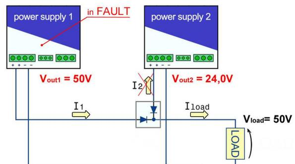
**Figure2** – System of 2 redundant power supplies: one of them was in failure in the  $V_{out}$  control, and  $V_{out}$  rises
