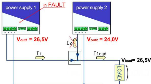
**Figure3** – System of 2 power supplies in redundancy: one has a fault in the control of  $V_{out}$  that cause the increase of  $V_{out}$ , but the power supply is equipped with overvoltage protection on the output.
