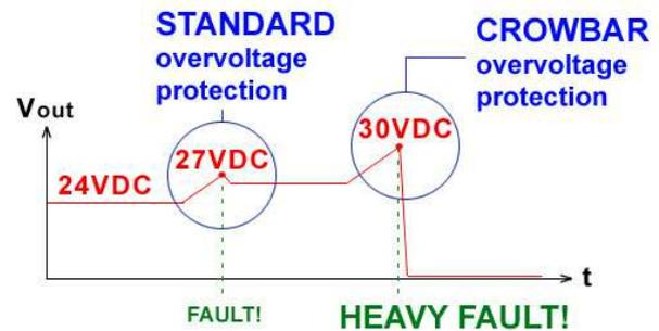
**Figure4** – Example of a standard overvoltage protection intervention, and CROWBAR intervention in an Advel SPS series power supply, output rated 24VDC
