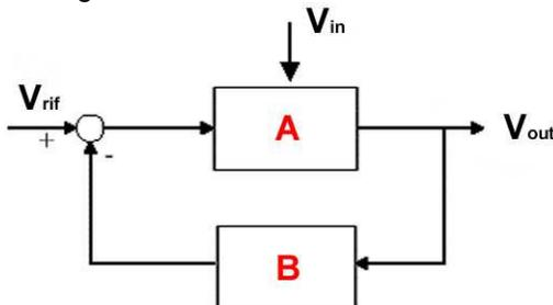
**Figure1** – Block diagram for a feedback system, which can be applied to the control of  $V_{out}$  in a stabilized power supply
