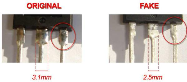
Figure7 – Detail of the legs of the two components
