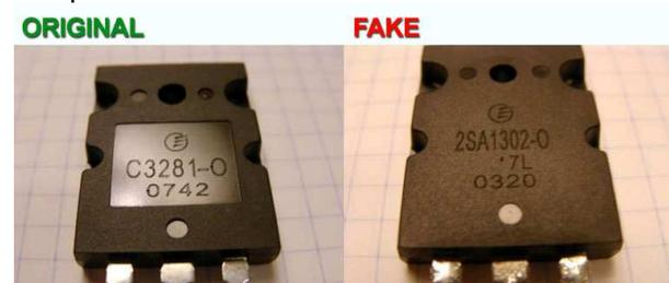
Figure1 – Two transistors: on the left the original, on the right the counterfeit one.
