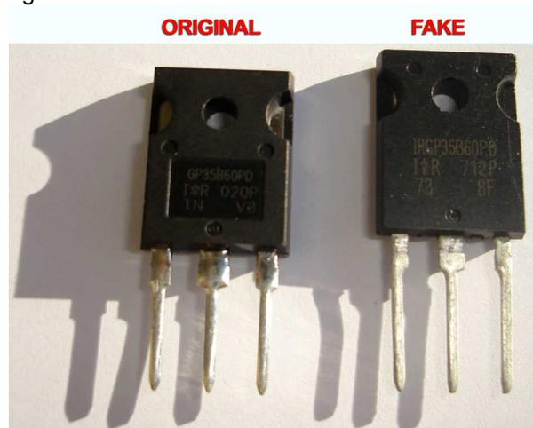
Figure5 – Two IGBTs IRGP35B60PD: the original one on the left, the conterfeit one on the right.
