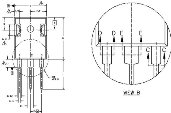
Figure6 – Dimensioned drawing of the component (image taken from the original manufacturer's datasheet)
