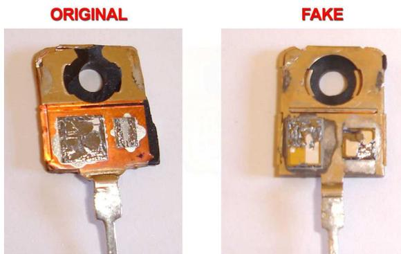
Figure8 – The two IGBTs have been "opened": the size of the junctions and the underlying metallization is a proof that the two components followed a very different production process.
