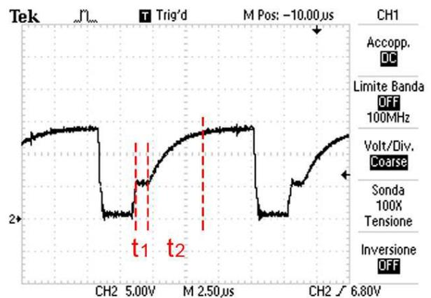
Figure9b –  $V_{be}$  of the fake IGBT
