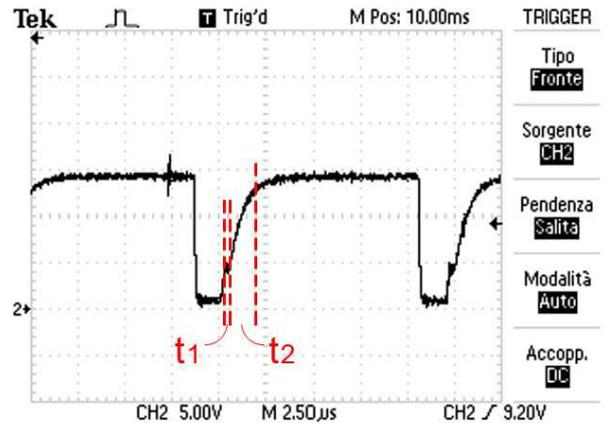
Figure9a –  $V_{be}$  of the original IGBT
