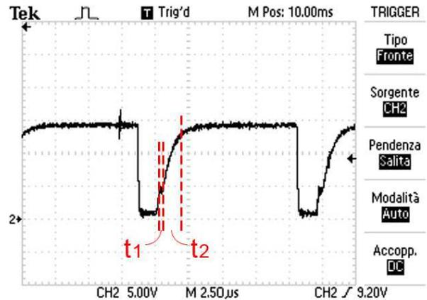
Figure9a –  $V_{be}$  of the original IGBT
