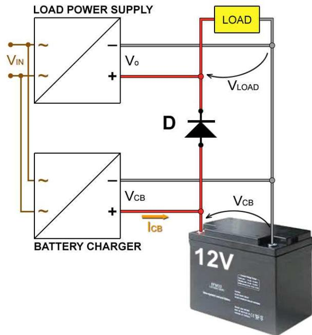
**Figure2** – Simplified Stand-by DC-UPS system: the power supply for the load and the charger are decoupled by a diode instead of a switch.
