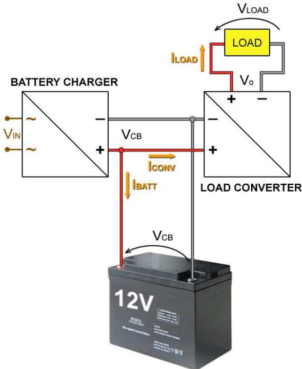
**Figure3** – Online DC-UPS system composed of a battery charger and a DC/DC converter.
