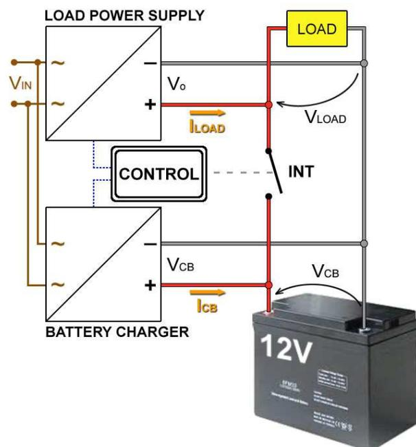
**Figure1** –Stand-by DC-UPS system composed of: a power supply for the load and one for the battery.
