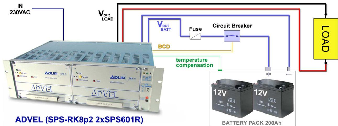
**Figure8** – DC-UPS system, realized with an Advel power supply (rack 19" SPS-R series, containing two hot-plug 600W modules, the SPS601R) with battery control and temperature compensation.
