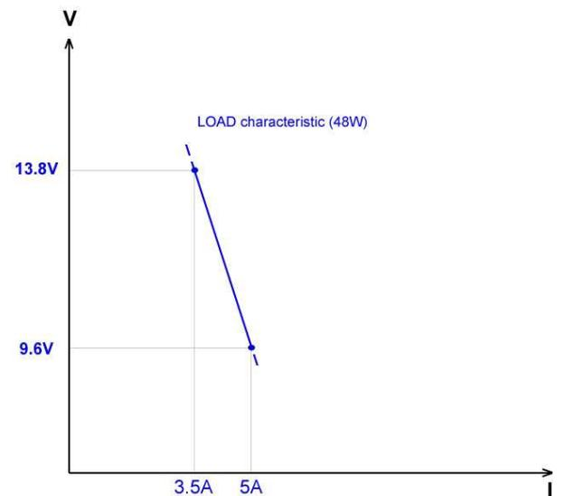
Figure6 – I/V characteristic of a "constant power" load, powered between 9.6V and 13.8V.
