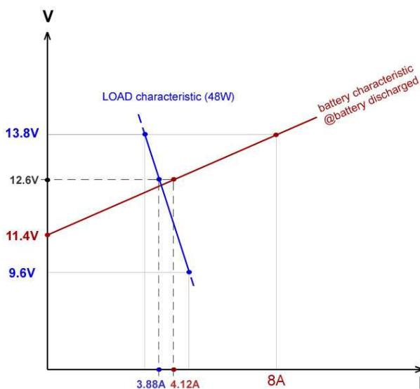
**Figure 7** – Graphical calculation to find the voltage such that  $I_{\text{batt}} + I_{\text{load}} = 8A$ .
