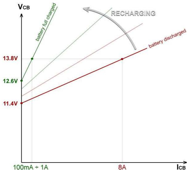
Figure5 – Qualitative characteristic I / V of a 12V-40Ah battery depending on the state of charge, @25°C.
