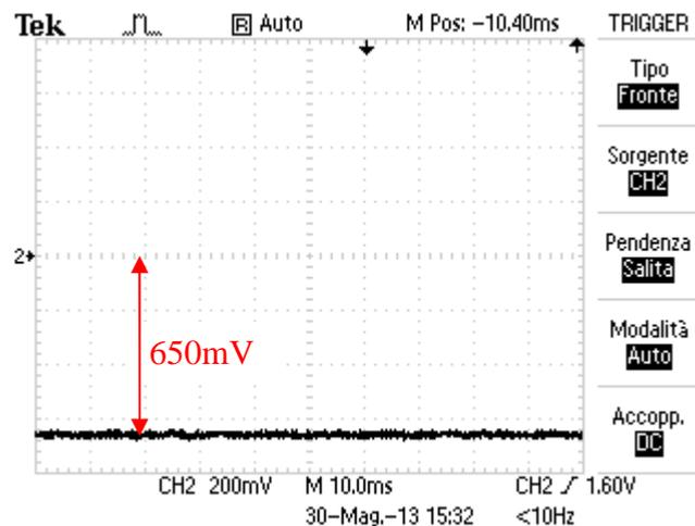
**Figure4A** –  $V_{fmA}$  for diode A, at 3A load current, @35°C.
