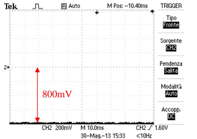
**Figure4A** –  $V_{fmA}$  for diode A, at 3A load current, @35°C.
