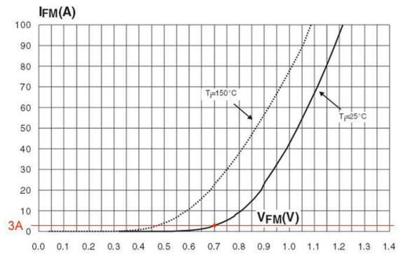
**Figure3** – Forward characteristic  $V / I$  of the diode (taken from ST datasheet). Pointed out in red 3A load.
