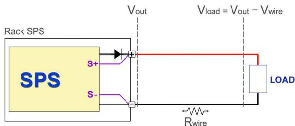
Figure4 – In a standard SPS system, voltage sensing takes place on the output terminals of the rack. The voltage on the load is equal to  $V_{out} - V_{wire}$  (NOTE:  $V_{wire}$  = voltage drop on the connecting cables).
