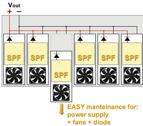
Figure3 – HOT SWAP of SPF modules, which also contain the fans and the decoupling diodes.
