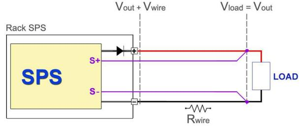
Figure5 – In an SPS system with **Sense Remote** option, the voltage sensing is brought directly to the load, to compensate the  $V_{wire}$ .
