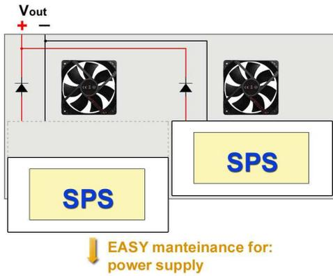
Figure2 – HOT SWAP of SPS modules, however the fans and the decoupling diodes are not easily replaceable.
