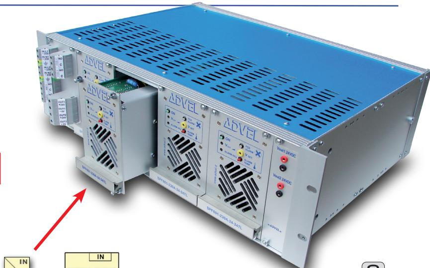
The modules let the hot plug-in/out, greatly simplifying installation and maintenance phases.
