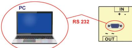
Standard RS232 Communication Port, to connect with a personal computer or supervision and data acquisition system.
